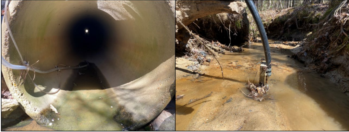
Figure 4. Monitoring setup of bubbler and sampler tubing in pipe (left) and channel (right)
